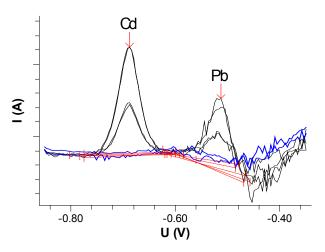
Determination of cadmium and lead by anodic stripping voltammetry at a mercury film electrode
