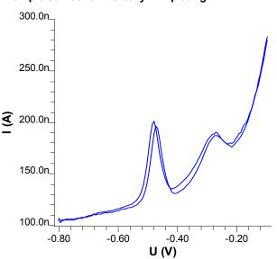
The peaks at -0.5 V and -0.3 V are related to lead and copper contamination of the Hg plating solution. These signals increase the more often the solution is used.
