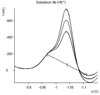
The shoulder at - 980 mV is caused by approx. 250 μg/L Zn Standard addition curve: Mo
