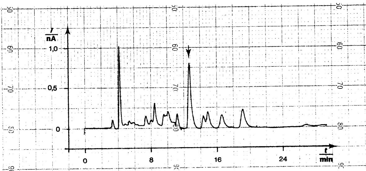
**HPLC/ELCD-Application****Substance****Phenols in wastewater**
