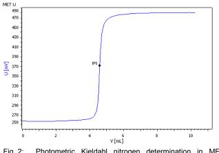
Fig. 2: Photometric Kjeldahl nitrogen determination in MET modus
