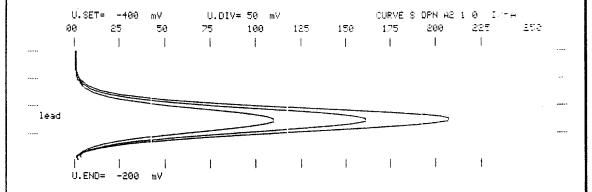
Determination of lead in "red" fuel: Program of the 646 VA Processor for the determination of the blank value in  $\mu g/L$  (or for "green" fuel)
