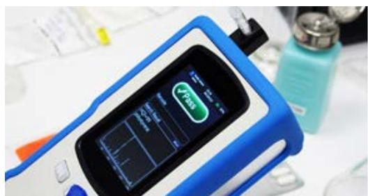
One of the most accomplished of these compact, hand-held Raman spectrometers for the inspection of raw materials and chemicals is the NanoRam® (B&W Tek, Newark, DE, USA). The NanoRam is a state-of-the-art, hand-held Raman spectrometer weighing just 1 Kg (2.2 pounds) for material identification and verification within regulatory-compliant environments. Designed
