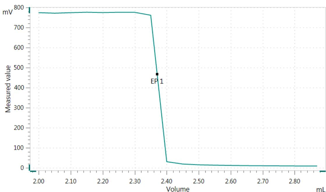
The bromine number is an important parameter for the determination of aliphatic C=C double bonds in petroleum products. The bromine number is usually determined using electrochemical titration at 5 °C, where the bromine is generated in situ from a bromide/bromate solution. For the titration, a solvent mixture of glacial acetic acid, methanol, and chloroform is used. In this Application Note, the toxic chloroform was replaced with diethyl carbonate.
