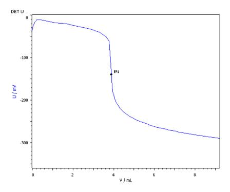
Mercaptans in refinery products can be determined by potentiometric titration with silver nitrate. This Application Note describes their automatic determination in a gas oil sample.
