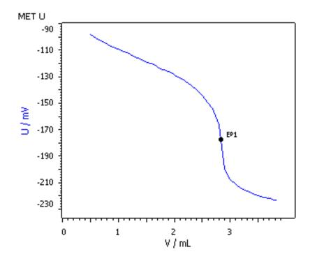
Magnesium can be analyzed using the Cu ISE. A small amount of Cu-EDTA complex thereby acts as indicator as the Cu ISE itself is not sensitive for magnesium.
