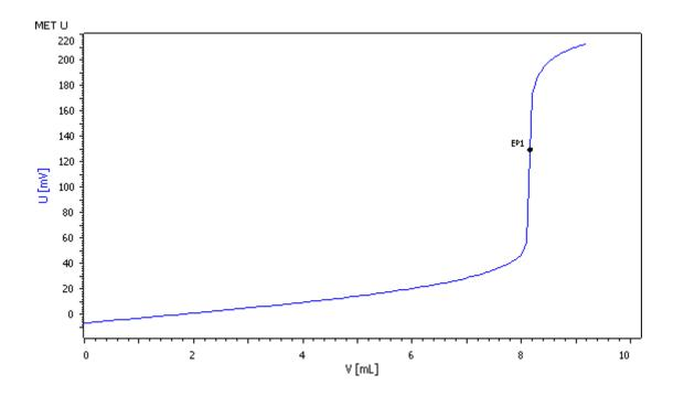
This Application Note describes the fully automated complexometric determination of aluminum in aqueous solutions with a copper ion-selective electrode and the MATi 07 system.
