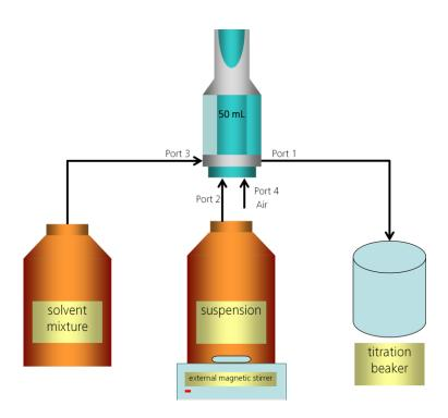
Automated mixing of a suspension and a solvent in a 50 mL Dosing unit can be used to add a well-defined amount of a suspension to a sample solution without clogging the dosing unit and tubing by the undiluted suspension.
