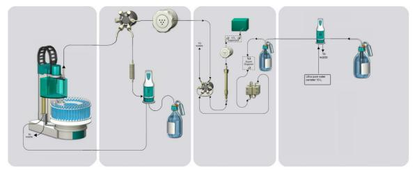
System setup: Sample Processor with rinsing station, diversion valve, 800 Dosino for liquid handling with transfer tubing, Sample Preparation Module (SPM), IC system with 250  $\mu$ L loop for MiPT, and inline eluent preparation.
