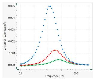
Figure 3 – Imaginary component -Z"(IMVS) of the IMVS transfer function plotted versus the frequency at 5 mW/cm² (blue dots), 10 mW/cm² (red dots), and 50 mW/cm² (green dots).
