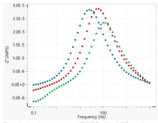
Figure 6 – Imaginary component -Z"(IMPS) of the IMPS transfer function plotted versus the frequency at 5 mW/cm $^2$  (blue dots), 10 mW/cm $^2$  (red dots), and 50 mW/cm $^2$  (green dots).
