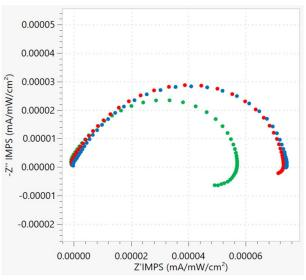
Figure 5 – IMPS measurement obtained at 5 mW/cm² (blue dots), 10 mW/cm² (red dots), and 50 mW/cm² (green dots).
