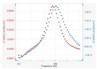
Figure 7 - Comparison of the -Z" versus frequency plots for IMPS (blue dots) and IMVS data (red dots), obtained at 50 mW/cm<sup>2</sup>
