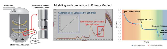
Stylization of suggested placement for NIR probe in an industrial PU reactor with real data correlation between primary titration method and NIR model showing how different mixing steps can be shortened.
