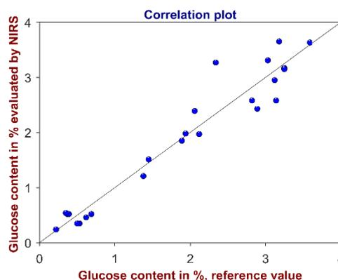
Fig. 2: Validation of the method for the determination of glucose content. The correlation plot shows reference values versus glucose values evaluated by Vis-NIR spectroscopy. High coefficient of determination ( $R^2 = 0.9623$ ) and low standard error of prediction ( $SEP = 0.34\%$ ) demonstrate that the method is suitable for its intended use.
