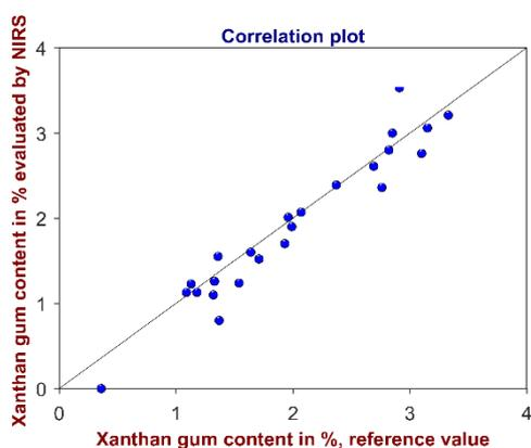
**Fig. 3:** Validation of the method for the determination of xanthan gum content. The correlation plot shows reference values versus xanthan gum values evaluated by Vis-NIR spectroscopy. High coefficient of determination ( $R^2 = 0.9431$ ) and low standard error of prediction (SEP = 0.35%) demonstrate that the method is suitable for its intended use.
