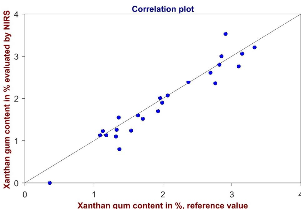
Near-infrared spectroscopy (NIRS) was used as an analysis method for quality control of aqueous xanthan gum solutions. Quantitative models for the determination of optical density, glucose, and xanthan gum were developed, enabling fast and reliable quality control.
