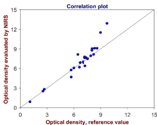
**Fig. 4:** Validation of the method for the determination of optical density. The correlation plot shows reference values versus optical density values evaluated by Vis-NIR spectroscopy. High coefficient of determination ( $R^2 = 0.9052$ ) and low standard error of prediction (SEP = 0.90) demonstrate that the method is suitable for its intended use.
