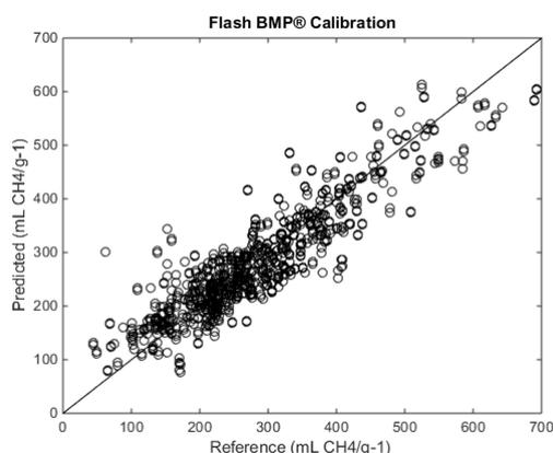
Fig. 2: The correlation plot of the PLS regression of the samples from the Flash BMP<sup>®</sup> calibration model.
