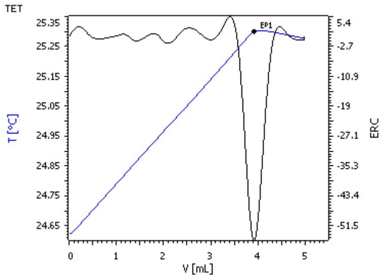
*Fig. 2. Titration of sulfuric acid component with  $c(\text{BaCl}_2) = 1 \text{ mol/L}$*
