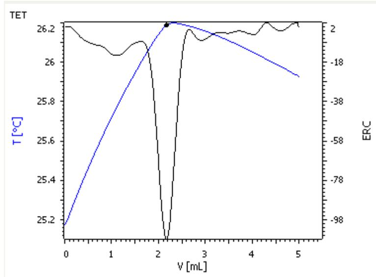
*Fig. 1. Thermometric titration of total fluoride concentration with  $c(\text{Al}(\text{NO}_3)_3) = 0.5 \text{ mol/L}$*
