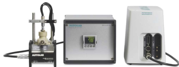
Figure 1 - The Autolab Microcell HC combined with the Metrohm Autolab PGSTAT204 with FRA32M module.
