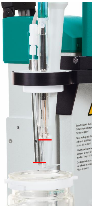
Figure 5: The pH electrode and the conductivity measuring cell are placed at different heights because the immersion of the electrode into the water may affect the conductivity. By considering this, the pH electrode is not immersed into the water during conductivity measurement.
