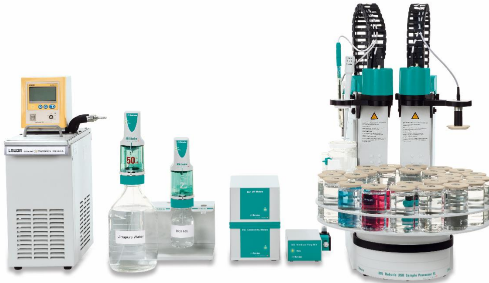
Figure 4: Overview of the whole system for water analysis consisting of a thermostat, a 867 pH module, a 856 conductivity module, an 815 Robotic USB Sample Processor XL, an LL-Aquatrode plus and a conductivity measuring cell. The left swing arm is used for analysis and the right one for the DIS-Cover
