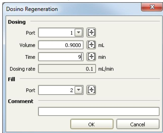
If you alter these parameters, be careful to choose the dosing time about 1 min less than the automatic stepping time. This needs to be chosen in order to give the Dosino time to refill before the next dosing step. The regeneration dosage is always triggered by the step of the MSM. The maximal dosing rate is set to 2 mL/min.
