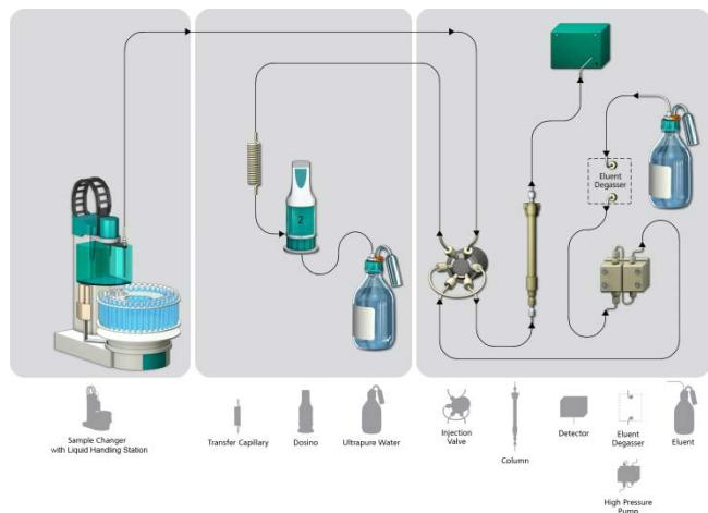
Prepare and degas an eluent suitable for column you want to use (see column manual). For Metrosep C 4 - 150/4.0 a solution of 1.7 mmol/L HNO<sub>3</sub> / 0.7 mmol/L dipicolinic acid (DPA, 2,6-Pyridinedicarboxylic acid) is adequate.
