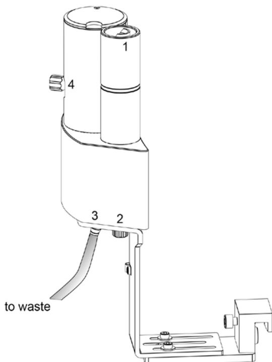
Number 4 of the picture above shows the attachment point of a capillary in case of a dilution feature and Number 1 indicates the rinsing entity.
