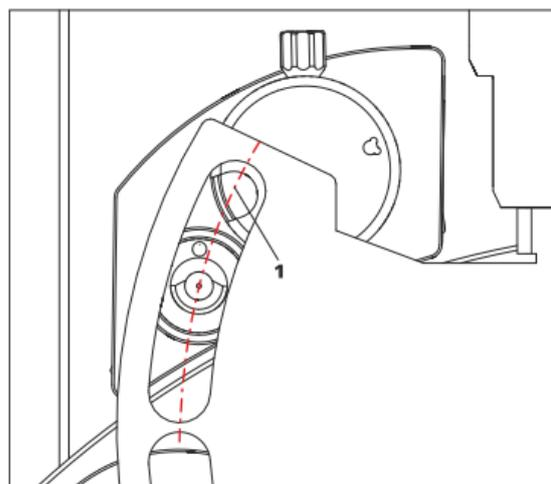
When you have found the correct position, please tighten the screw to fix the LQH Station completely to the Sample Processor.
