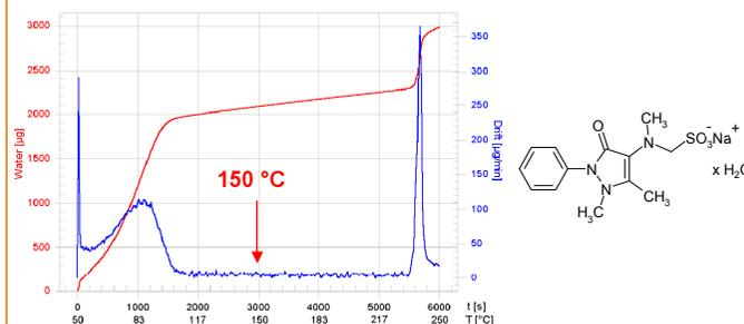
The water release curve was recorded using a heating rate of 2 °C/min.
