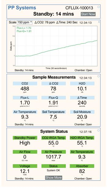
Sensor data and information is easily viewed via computer or mobile device. Flux rates based on linear and quadratic fit are continuously calculated and displayed.
