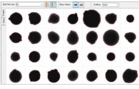
Particle images of metal powder which are used for Additive Manufacturing: Some particles have satellites, i. e. small particles fused to large ones.
