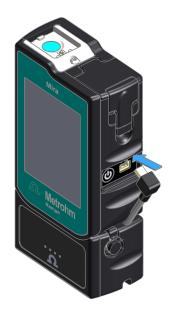
Connect the USB Mini-B plug to the instrument.
