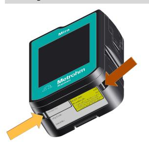
Remove the lanyard from the lanyard pins.
