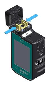
Open the Tablet Holder. Push the levers and position the sample in the middle.
