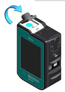
Attach the Smart Tip by engaging the bottom left corner of the tip into the left edge of the mounting point. Rotate the tip into position.
