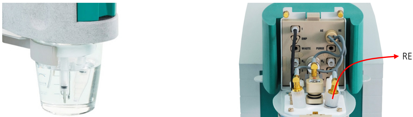
Figure 12: Electrode storage: a few hours in deionized water (left) or RE removed from measuring head, if not used overnight or longer (right)
