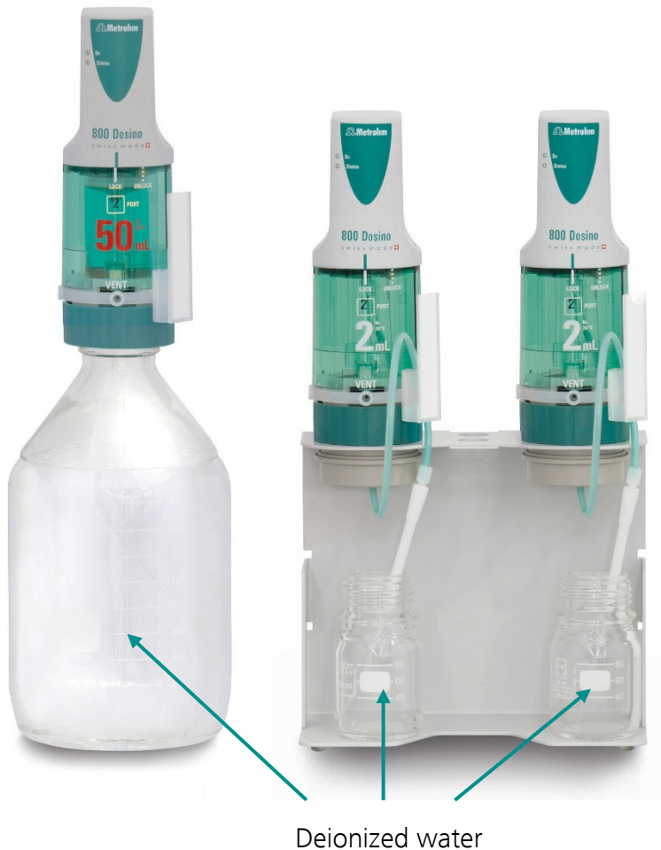
Figure 15: Preparation of the 807 Dosing Units with deionized water.
