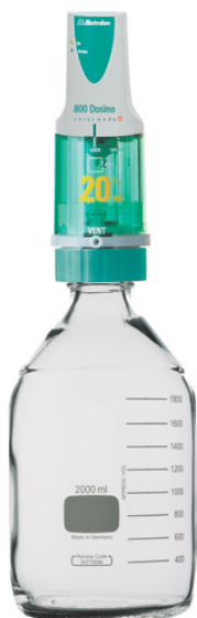
Figure 3 807 Dosing Unit with 800 Dosino and 2 L glass bottle
