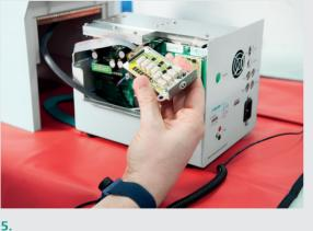
If necessary, the instrument will be opened in compliance with the directives for the prevention of ESD (electrostatic discharge), so as not to damage the highly sensitive electronic components.
