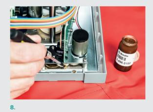
Moving parts require a fine film of grease in order to operate with the least possible friction and wear. Applying a **lubricant and/or grease** is an integral part of any regular preventive maintenance.
