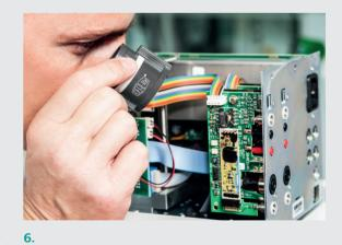
The Metrohm service engineer will perform a thorough cleaning of the interior of the instrument. Next, a thorough visual inspection will be made of the mechanical and electronic components and cabling. Particular attention will be paid to potential damage by any liquids that may have leaked into the instrument.
