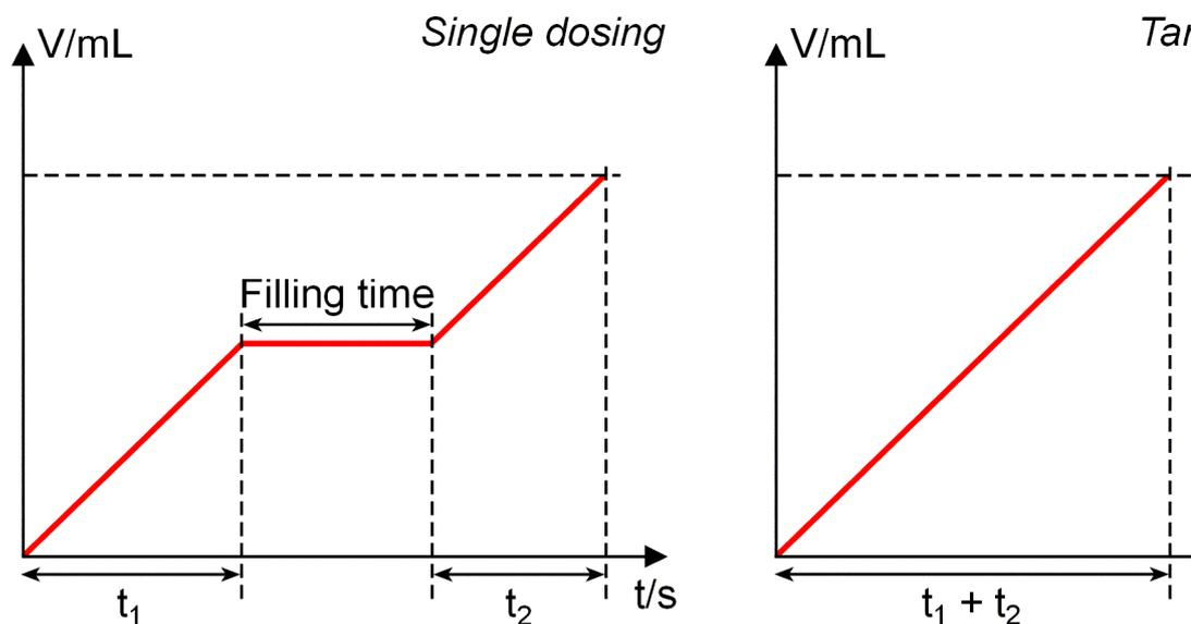
The time defined under dosing time corresponds to the net dosing time  $t_1+t_2$ , i.e. the filling time of the exchange/dosing unit is not included in the total.
