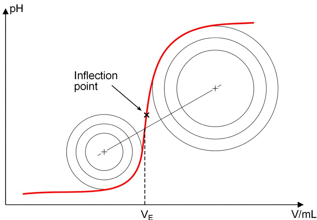
The figure shows that the evaluation still requires measured values from the measuring point list also after the equivalence point.
