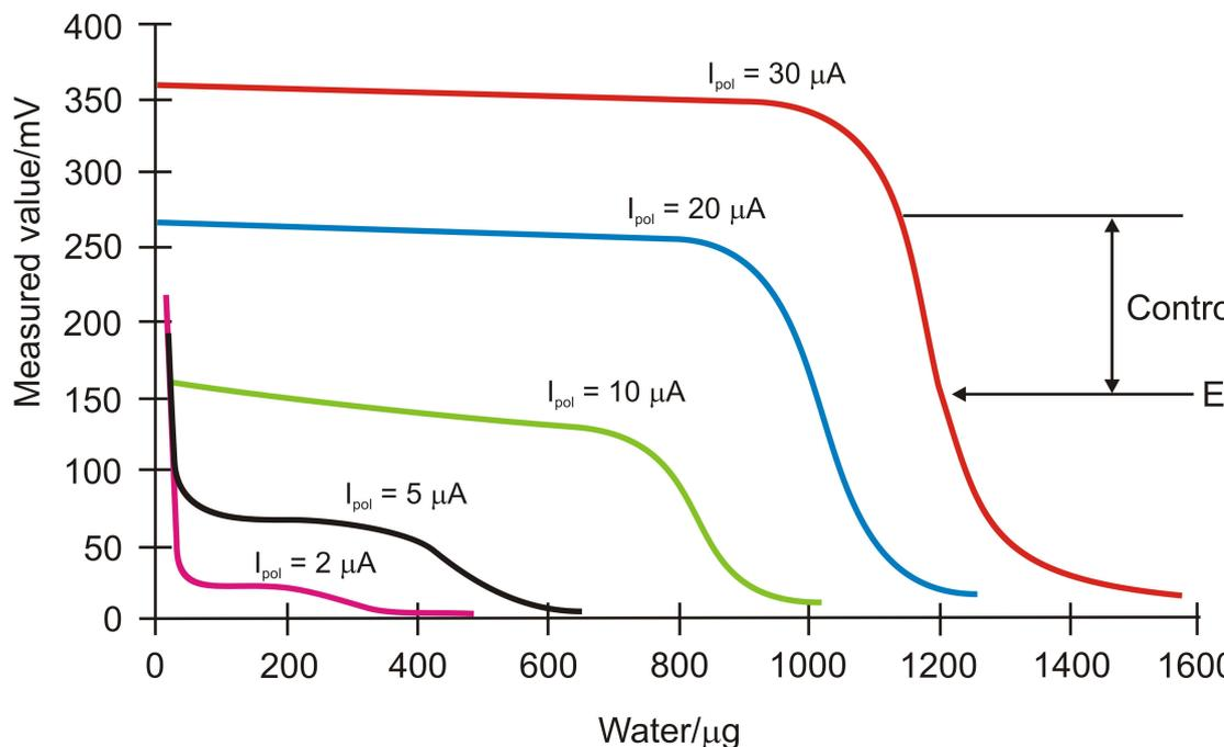
The diagram shows KF titration curves at different polarization currents. It is clear to see that the position of the endpoint varies with the polarization current. The curves have different slopes, i.e. the dynamics must also be adapted. Polarization currents smaller than 10  $\mu\text{A}$  are not suitable for this application. The following table gives an idea of the optimal control parameters for various polarization currents.
