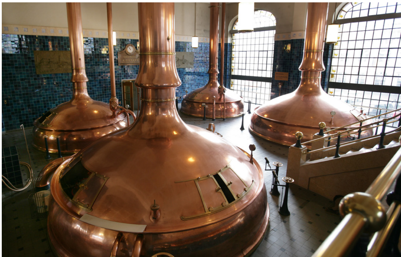
Figure 3. The wort is still boiled in copper wort kettles in the Art Nouveau brewhouse which was built in 1909. This process causes the \alpha -acids in the hops to isomerize into iso- \alpha -acids.
