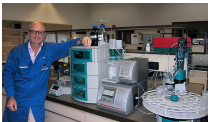
Figure 2. Jules Wyss with his analysis system in the quality assurance laboratory at Feldschlösschen in Rheinfelden. The system combines ion chromatography, titration, density measurement, and spectroscopic alcohol determination.
