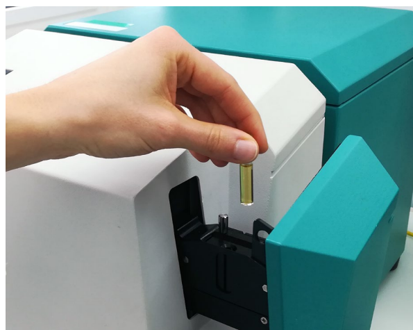
Figure 1. XDS RapidLiquid Analyzer and an isocyanate sample present in the 8 mm Disposable Vial.
