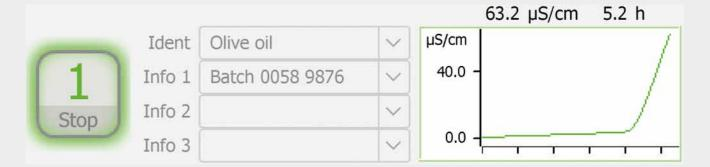
For each measuring position on the instrument there is a live display in the «Workplace» part of the program. The flashing Start/Stop button indicates a determination is running. From the corresponding live curve it is possible to see directly the current status of the determination and the already detected
