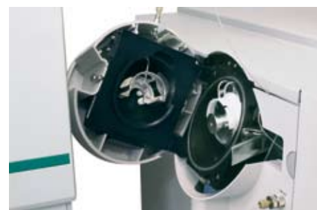
Close-up of the mass spectrometer's electrospray ionization (ESI) interface.
