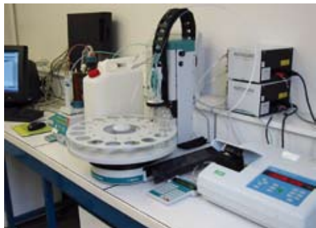
The completely automated water analysis system in the Laboratoire d'Analyses des Eaux des Yvelines.
