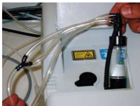
The flow-through cell of the Hach 2100AN IS Turbidimeter.
